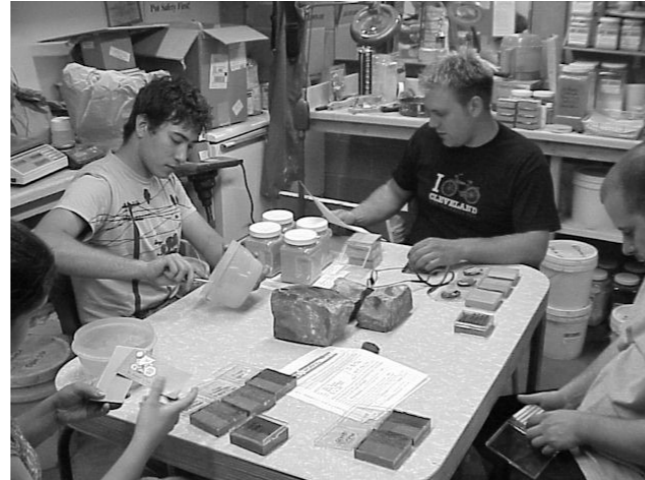
From lower left corner to right: Anya, Randy, Mike, and Phil began their work at Andy’s lab. Prior to any work on the site, much of the preparation takes place in the lab. After taking multiple mortar and stone samples, the apprentices were given the job of creating mortars and stone patch samples that matched in color and texture to the original.
